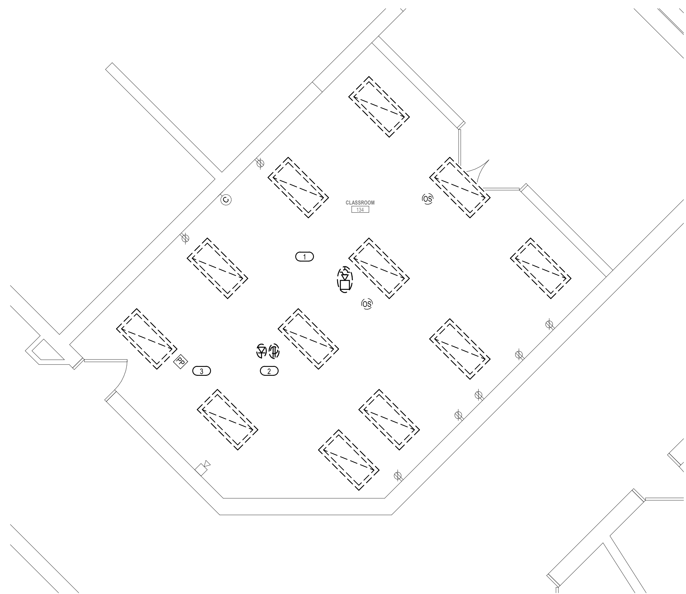
2 FIRST FLOOR ELECTRICAL DEMO PLAN AREA "C" 1/4" = 1'-0"
